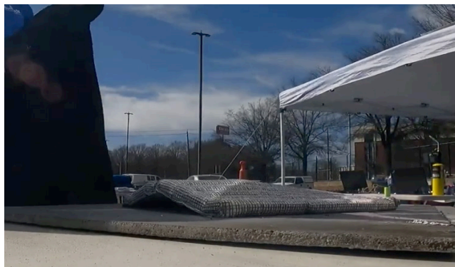
Application of PED-Pad fire suppression pillow and LIBIK fire blanket.
