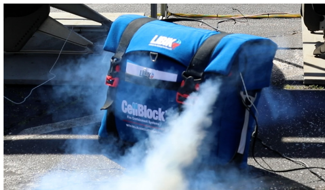
Test sample in thermal runaway. Explosion evident.
