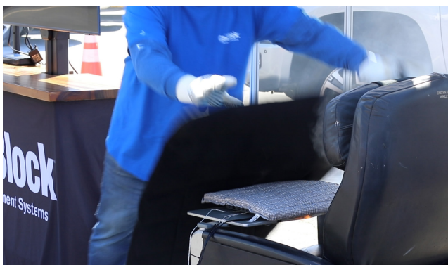
PED-Pad fire suppression pillow and LIBIK fire blanket application.
