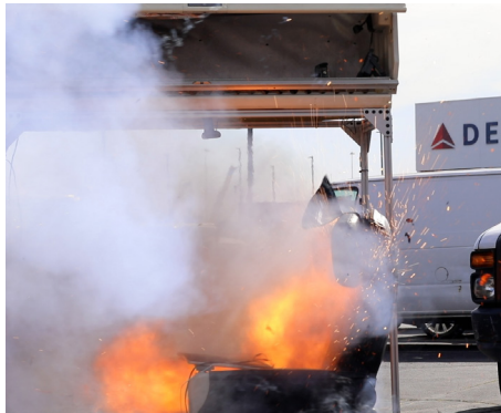
Test sample in thermal runaway.
