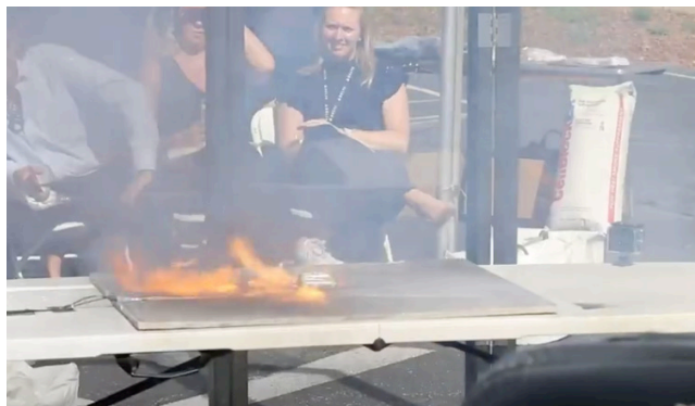
Test sample in thermal runaway.
