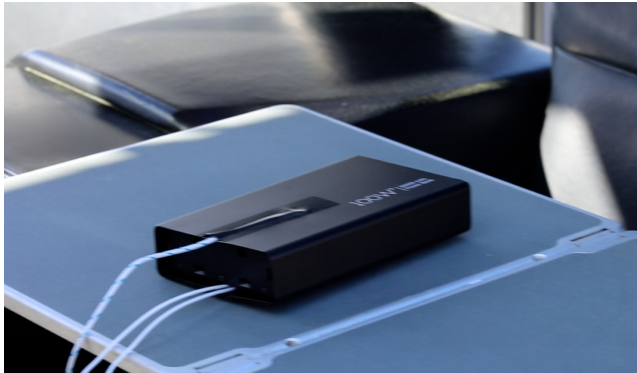
Test sample pre-test - 74 Wh consumer battery pack
