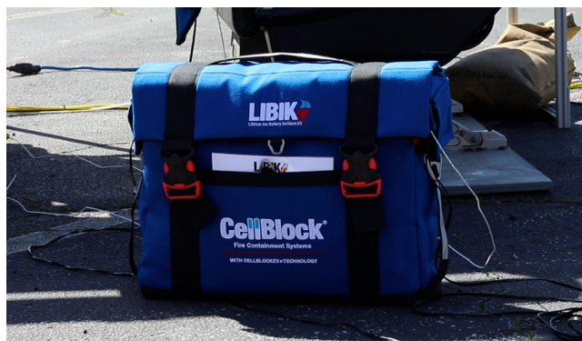
Test sample pre-test - power bank placed in LIBIK kit
