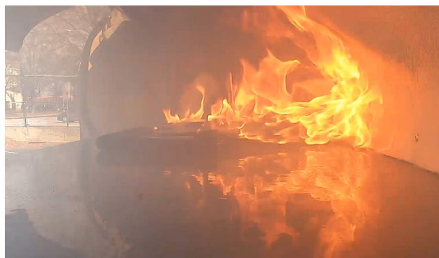
Test sample in thermal runaway.
