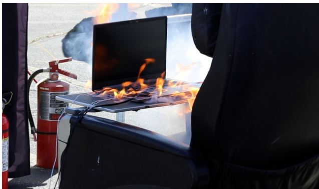
Test sample in thermal runaway.
