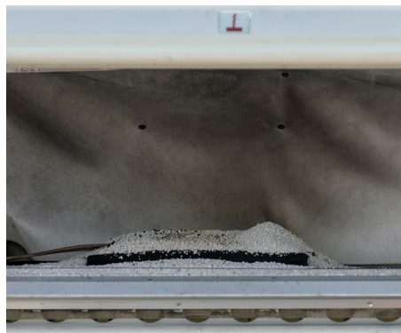
Overhead bin, post test. Cells fully extinguished.
